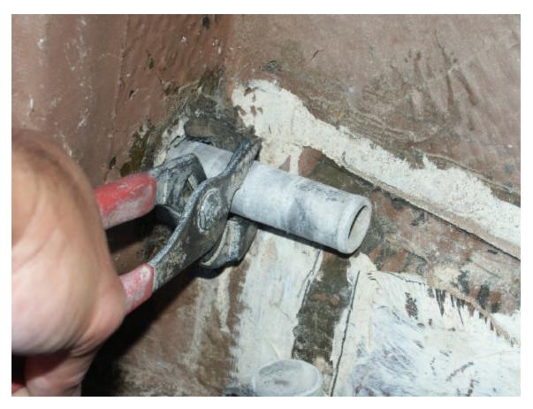
Removing pipe. (Turn and pull pipe through hull. You may need another person at other end to tap pipe with hammer and punch to push pipe through and disengage from through-hull on opposite side.)
