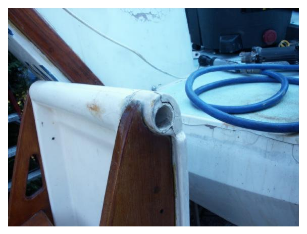
Swim step removed (with pipe removed). Pipe slides out of swim step.
