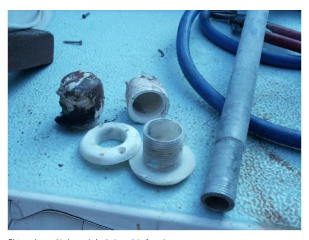
Picture shows old pipe and plastic through-hulls and cap.
